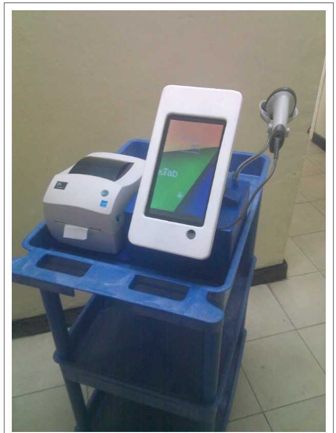
FIGURE 1: A mobile workstation equipped with a tablet computer, label printer and barcode scanner, Kamuzu Central Hospital, Malawi, 2015.
